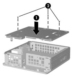
Figure 2-7 Replacing the metal side cover
